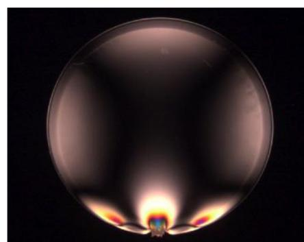
LSM-8000LE visualize a inside stress or birefringence in a transparent material by using polarization technique. This product is suitable for big sample.
