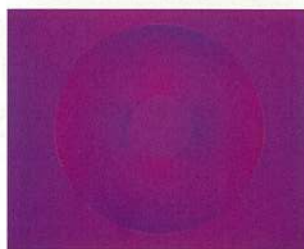
Sensitive Tint Color Method Hard disk glass
