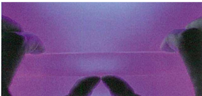
Stress-direction-determining bar with no strain
