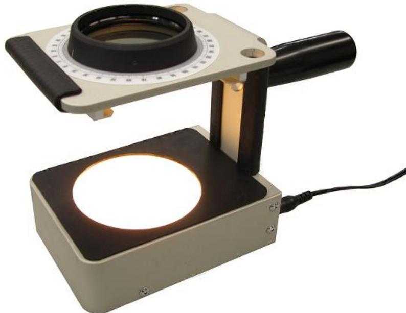
LSM-1000LE visualize a inside stress or birefringence in a transparent material by using polarization technique. It is possible to analyze the optical direction or quantify the retardation relative to inside stress if optional sensitive tint plate or 1/4 wavelength plate is attached to the equipment. It is compact and lightweight. AC adapter is included as standard. Optional battery unit for carrying around and using is prepared.
